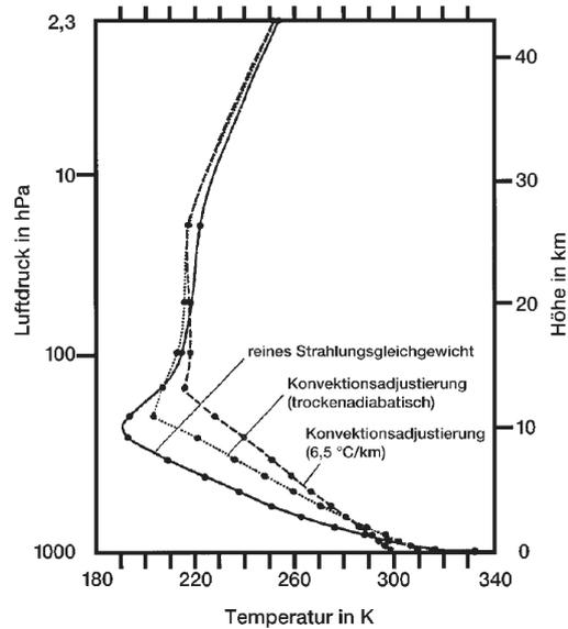
Figure 0: Temperature profile in the radiation balance without (solid line) and with adjusting of the convection on dry adiabatic temperature (dotted line) and observed mean lapse rate of 6.5°C/km (dashed line), calculated by MANABE und STRICKLER (1964). (From [36, Abb. 2-5])
