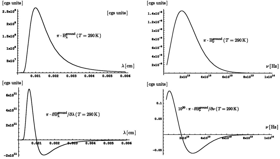
Figure 9: The radiation intensity of the ground and its partial derivative as a function of the wave length (left column) and of the frequency (right column).
