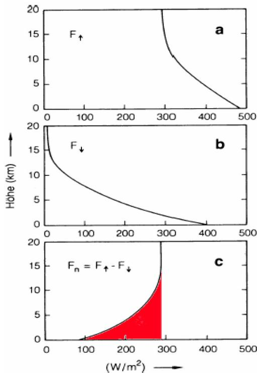
Figure -1: Radiation intensity upward (a) and downward (b) and the difference of both (c - net radiation flux). The image c is added with the convective heat (red area). (From [210, Abb. 1.22, S. 47])
