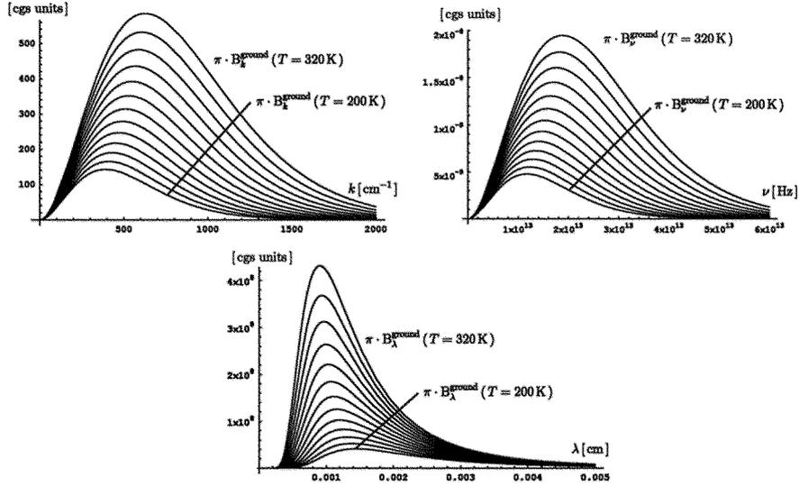
Figure 10: Three versions of radiation curve families of the radiation of the ground (as a function of the wave number  $k$ , of the frequency  $\nu$ , of the wave length  $\lambda$ , respectively), assuming that the Earth is a black radiator.
