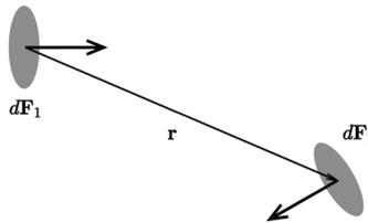
Figure 1: The geometry of classical radiation: A radiating infinitesimal area  $dF_1$  and an illuminated infinitesimal area  $dF_2$  at distance  $r$ .
