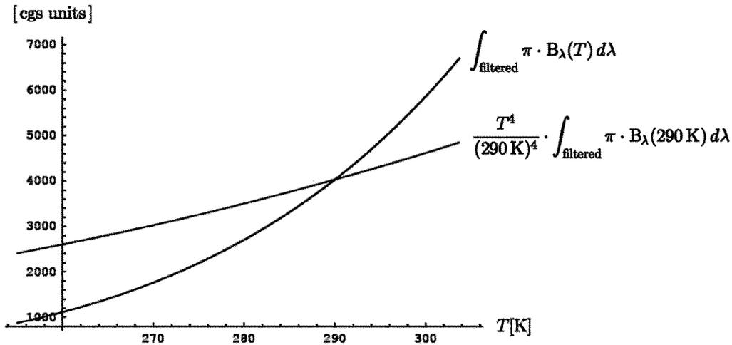
Figure 4: Black body radiation compared to the radiation of a sample coloured body. The non-universal constant  $\sigma$  is normalized in such a way that both curves coincide at  $T = 290$  K. The Stefan-Boltzmann  $T^4$  law does no longer hold in the latter case, where only two bands are integrated over, namely that of visible light and of infrared radiation from  $3 \mu\text{m}$  to  $5 \mu\text{m}$ , giving rise to a steeper curve.
